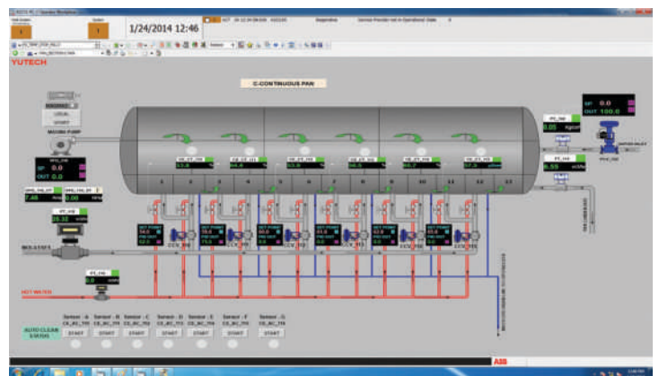
SCREEN SHOT: HORIZONTAL CONTINUOUS VACUUM PAN AUTOMATION
