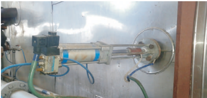
PICTURE OF YUTECH SELF CLEANING AUTO RETRACTABLE BRUX SENSOR INSTALLED ON CV PAN
