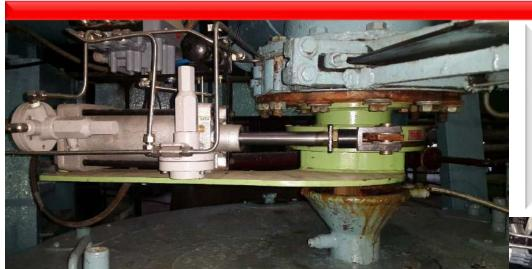
Controlled Quantity of Massecuite drops from the Concentric Opening (Split opening from the Centre of the Valve) Hence No Spilling, No Splattering, No Unbalance, No Overflow, No Underfeeding
