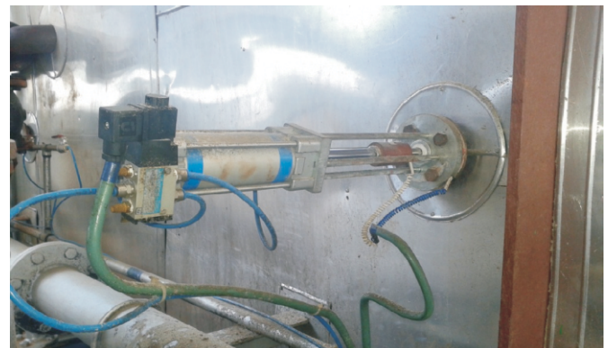
PICTURE OF YUTECH SELF CLEANING AUTO RETRACTABLE BRX SENSOR INSTALLED ON CV PAN
