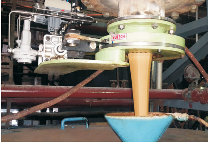
YUTECH CSD Valve also called Iris Valve based Automatic Feeding of Continuous Centrifugal Machine
