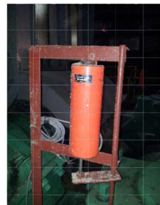
Mill Top Roller Lift Sensed Installation
