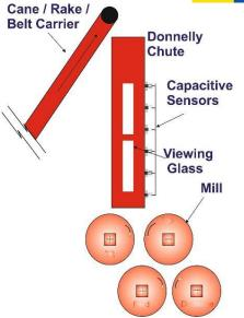
**BUILT-IN RAINING BAGASSE COMPENSATION**: TO ACCURATELY SENSE, ANALYZE, CALCULATE AND DERIVE ACCURATE CHUTE LEVEL WITHIN A VERY CHALLENGING ENVIRONMENT OF RESIDUAL JUICE DIRT, STICKY BAGASSE DUST AND VIBRATION
