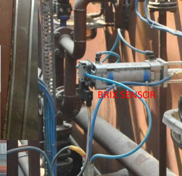
Auto Retracting Self Cleaning Brix Sensor installed on Continuous Vacuum Pan & Sugar Melter in Picture below
